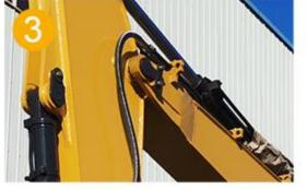
The link of the big and small arms is strengthened, the plate is thickened, the production process is improved, and the welding type is changed to an integrated casting type.
