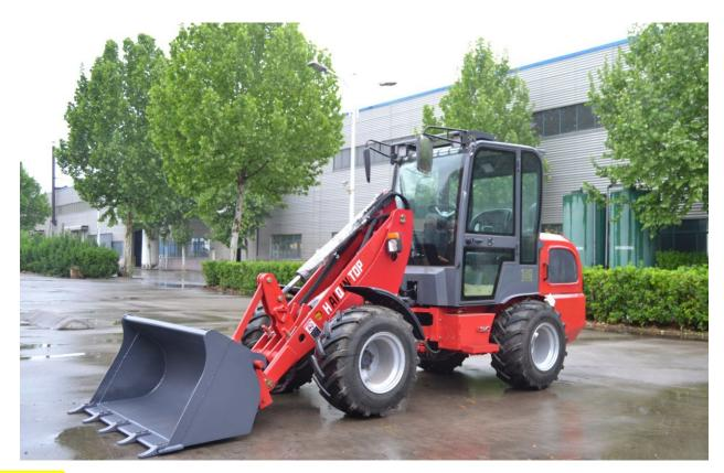
**Standard**: China changchai engine ,Mechnical Joystick, China hydraulic system,quick hitch, 31\*15.5-15 wide tire, closed cabin with heater, rear view camera, bucket etc.
